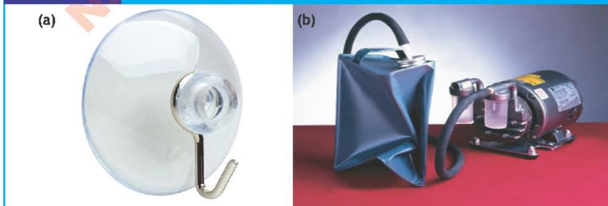
FIGURE 5.9 SUCTION CUP AND AIR EVACUATED FROM SEALED CAN
