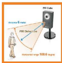
PIR Sensor used for detecting motion
