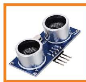
Ultrasonic Sensor for measuring distance
